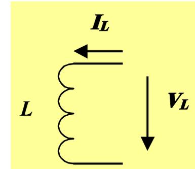
$$i(t) = i(t_0) + \frac{1}{L} \int_{t_0}^t v(t) dt$$
